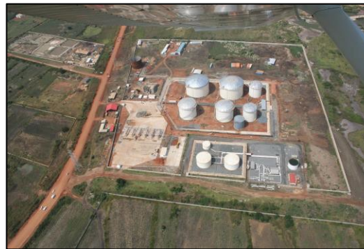
EPC for Clean Products Terminal for 90,000 Cubic Meters of storage, with in-bound pipeline system and truck racks – Tema, Ghana.
