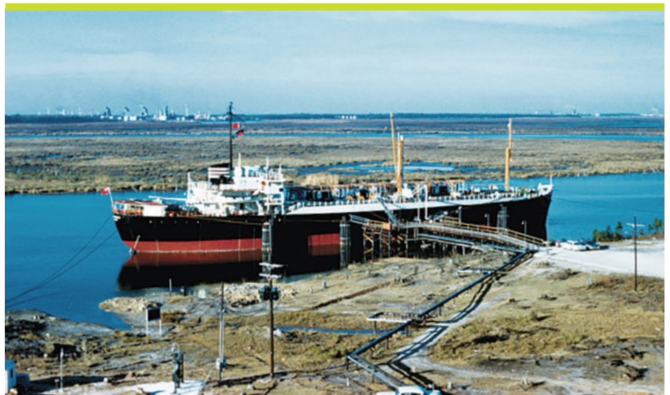
04 Methane Pioneer in Louisiana loading world's first export cargo of LNG bound for UK, January 1959
